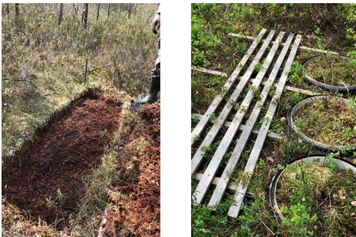
Figure 2.3.7. Gas measurement plots (heterotrophic respiration on left, total ecosystem exchange ( \text{CO}_2 , \text{CH}_4 , \text{N}_2\text{O} fluxes) in the right). Image: © G. Saule
