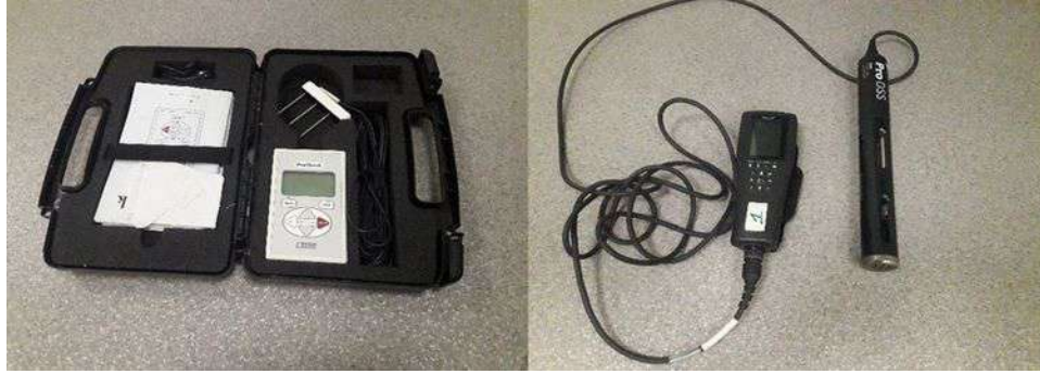
Figure 2.3.8. Equipment for measuring soil temperature, moisture content and groundwater properties. Image: © G. Saule
