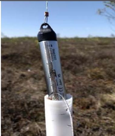
Figure 3.1.1 Installation of the groundwater level probe in Cena21 well in a 2006 restoration site with dens network of drainage ditches, May 7, 2024. Image: © A. Kalvāns
