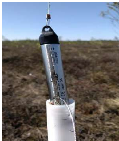
Figure 3.1.10 Installation of the groundwater level probe in Cena21 well in a 2006 restoration site with a dense network of drainage ditches, May 7, 2024. Image: © A. Kalvāns
