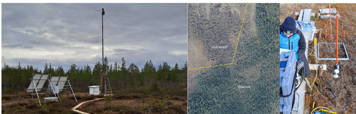
Fig. 12. Left) The eddy covariance measurement set-up for measuring \text{CO}_2 flux at Matorovansuo peatland. Middle) Drained and undrained source areas of the EC measurement. Data are attributed according to wind direction. Right) Chamber measurements were conducted in trenched and intact, vegetated points. The peatland type is a pine flark fen. Photos Jack Chapman, satellite image from National Land Survey of Finland 2023.
