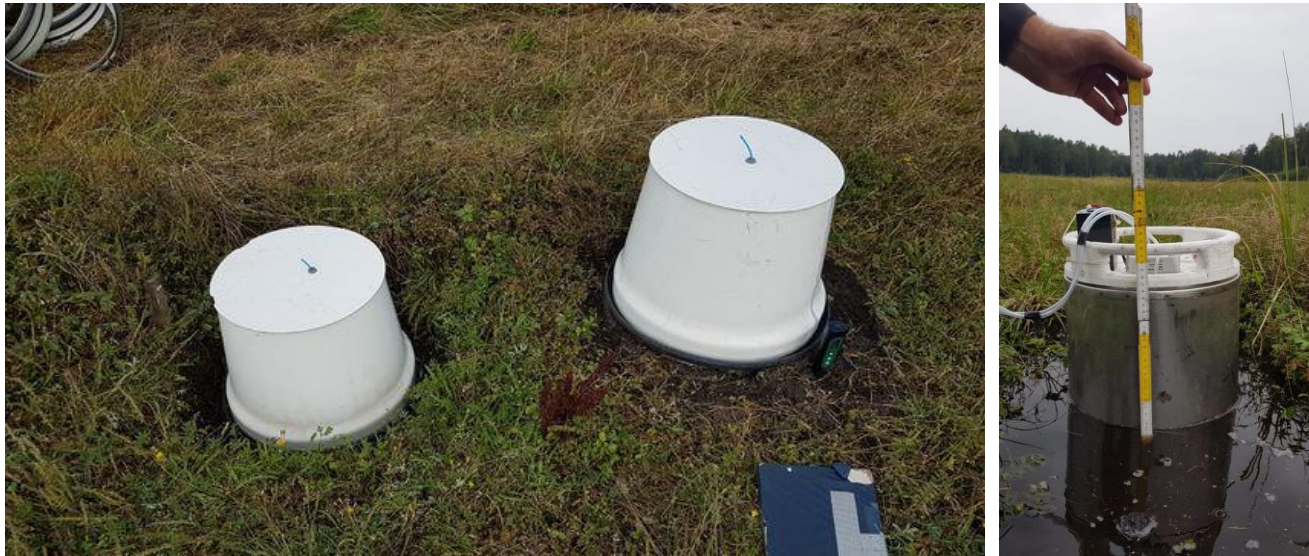
Figure 2.7. Gas measurement chambers (left) and soil heterotrophic measurement chamber (right).
