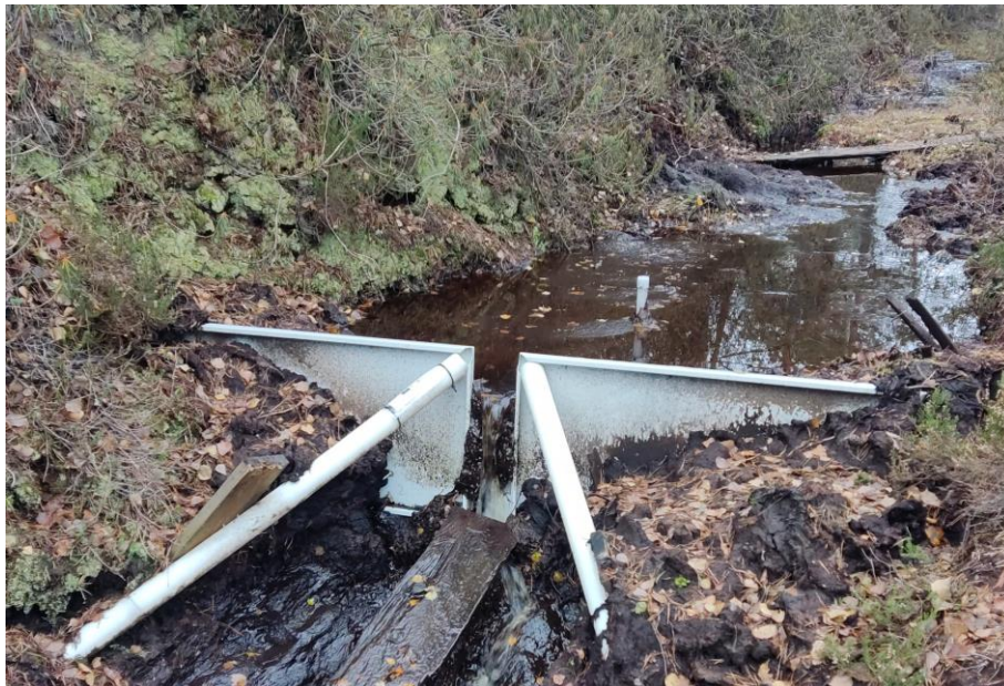
Figure 3.4. A discharge measurement spillway (monitoring point Cena8) clogged with eroded peat, November 10, 2023. Image: © A. Kalvāns
